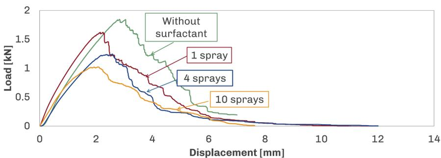
Figure 3 – Representative load-displacement curves for DCB tests for each contamination level
