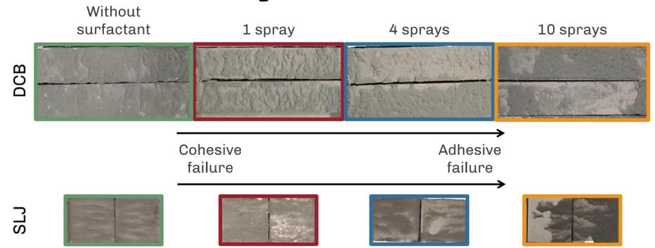
Figure 5 – Fracture surfaces for each contaminant level tested, for SLJ and DCB.
