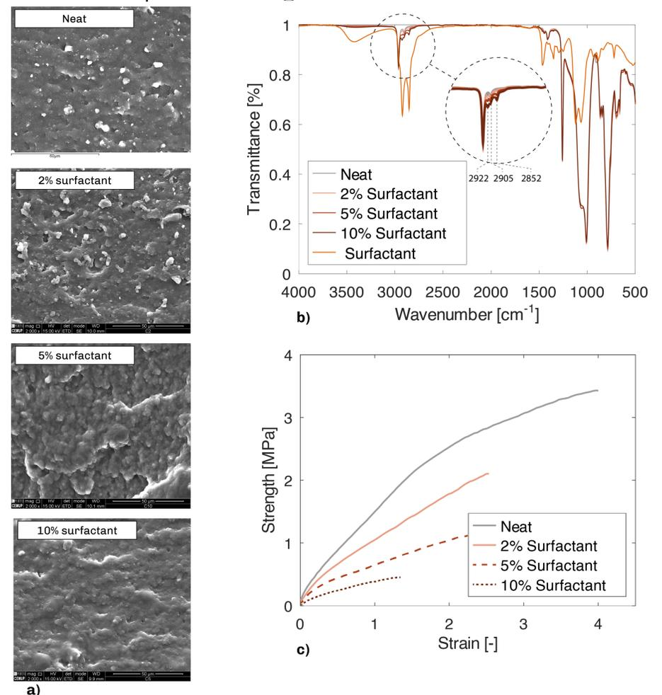
Figure 6 – SEM analysis a), FTIR analysis of the fracture surface b) and bulk tensile test results c).
